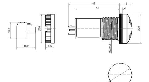
For additional installation and mounting information, refer to the appropriate user guide at www.werma.com. This printed copy is for information only and is subject to alteration.
